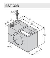
6947216 Mounting clamp for threaded barrel sensors, with dead-stop; material: PA6
