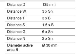
All non-flush mountable uprox®+ threaded barrel sensors can be screwed to the upper edge of the barrel. In this mounting position, the sensor operates safely with a 20 % reduced switching distance.
