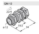
Quick-mount bracket with dead-stop; material: Chrome-plated brass. Male thread M16 × 1. Note: The switching distance of the proximity switches may change when using quick-mount brackets.
