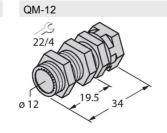
Quick-mount bracket with dead-stop; material: Chrome-plated brass. Male thread M16 × 1. Note: The switching distance of the proximity switches may change when using quick-mount brackets.
