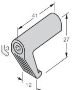
Mounting bracket for mounting magnetic field sensors on tie-rod cylinders; cylinder diameter: 63...160 mm; material: Die-cast Zinc
