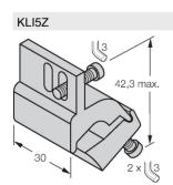
6971803 Mounting bracket for mounting magnetic field sensors on tie-rod cylinders; cylinder diameter: 32...63 mm; material: Aluminum
