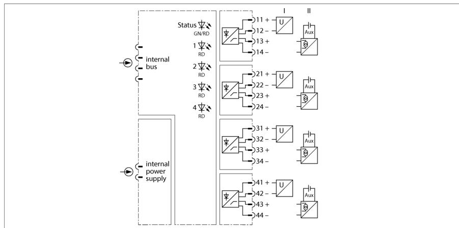
The input module AI41-N is used for the connection of 4-wire transducers (passive input = sink mode / transducer active).
