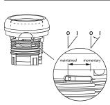
**Note:** Maintained pushbuttons can be converted in the field to momentary operation by switching the locking ring, which is accessible through the side of the operator body.
