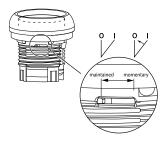
**Note:** Maintained pushbuttons can be converted in the field to momentary operation by switching the locking ring, which is accessible through the side of the operator body.
