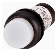
**Illuminated pushbutton actuator, Extended, momentary, 1 N/O, Screw connection, LED white, White, Blank, 230 V AC, Bezel: black**
