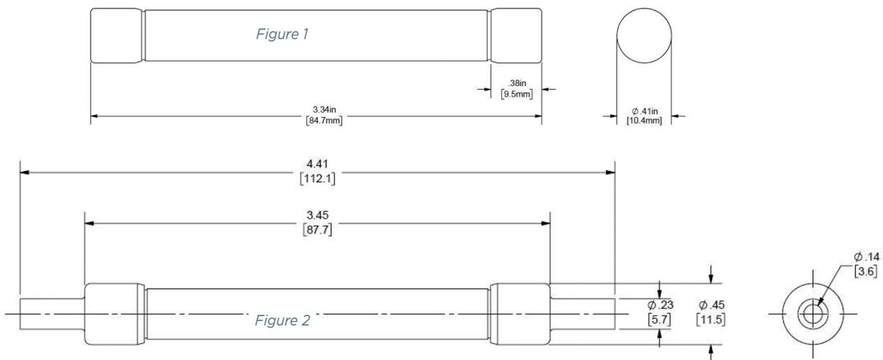
CC terminal (Fig. 2): Recommended crimping tool: T & B Sta-Kon ERG4002 #10 -12 AWG (6-4 mm<sup>2</sup>)
