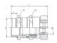
SKINTOP® GRIP-M is a double-strap strain relief cable gland with a high level of strain relief for harsh environmental conditions. Is is appropriate for portable equipment, cranes, conveying machinery, and systems on building sites.
