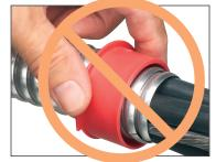
2 If you are using an end stop bushing, determine which one to use by sizing it to the cable bundle (not the metal jacket). Incorrect size shown above. The metal jacket should never go through the end stop.
