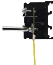
The screws can be tightened easily with a pneumatic screwdriver.
