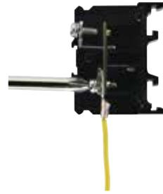
3. When the wiring is in position, tighten all the screws simultaneously.
