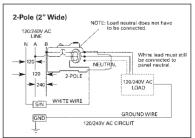
All BQ/BQH/HBQ circuit breakers are supplied with load side lugs. If line side lugs are required, add suffix "L" to catalog number. Consult Siemens for any additional charge. All standard circuit breakers are calibrated for 40°C maximum ambient application.
