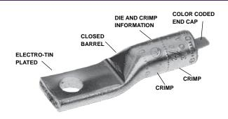
NOTE: Field bending straight lugs to achieve an angular connection will void UL Listing / CSA Certifications and BURNDY will not be liable for the connection.
