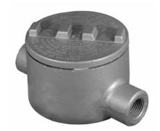
In Class I, Division 1, Group B atmospheres, all conduit runs must have a sealing fitting (not supplied) field-installed within 2" to the enclosure.
