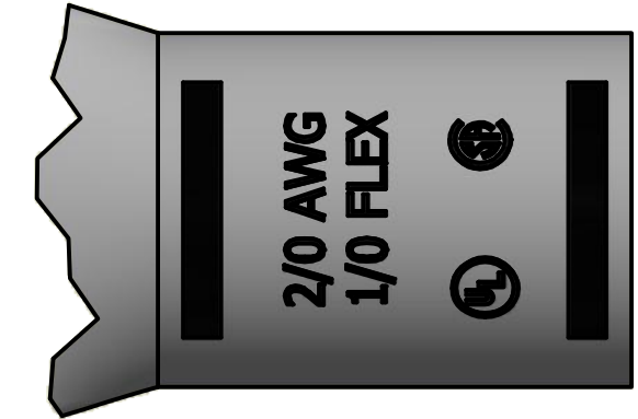
DETAIL E BOTTOM INK MARKING
