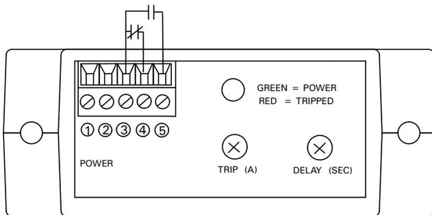
Current Sensing Switch Connections
