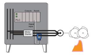
If the crusher drive draws to much current, the infeed belt can be stopped automatically, allowing the crusher to clear before restarting. The ASXP-MS also has a set of relay contacts for alarm of over or undercurrent conditions.
