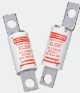
Mersen 2CL Cable Protectors are special purpose limiters which are crimped or bolted to cables or terminals to clear and isolate faults quickly, increasing the reliability of service entrance and distribution runs. They are 250VAC current limiting with a 200,000A interrupting rating, yet will carry low cable overloads which are handled by standard protective devices. These cable protectors are rated for both copper and aluminum cabling per their corresponding cable size.
