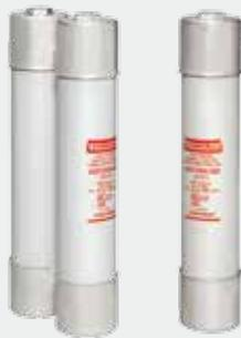
Mersen fuses for the protection of transformers and distribution lines deliver overload and short circuit protection. These current-limiting fuses will melt at current that can be as low as 1.7 times the fuse current ratings up to its maximum interrupting rating. These fuses are designed to withstand the transformer magnetizing inrush current. They have 2 (size C), 3 (size D) and 4 (size E) inch diameter barrels with ferrules and are mounted in spring reinforced clips.
