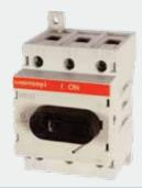
The M-series Load Break Switch is the most compact industrial-grade switch on the market. Capable of making or breaking loads up to 600V (UL), it is suitable as a motor disconnect. Extremely compact and robust, these switches have a variety of mounting options including DIN-rail, base, or door-mounting. A wide assortment of handles, shafts and accessories is available to accommodate any installation requirement.
